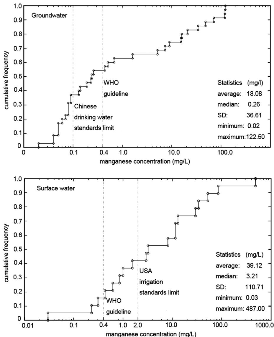
Fig. 2. Cumulative manganese distributions over wells and ponds.
