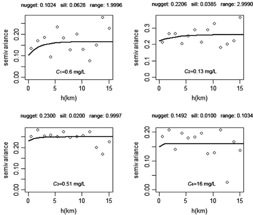
Fig. 3. Experimental variograms of indicator variables.
