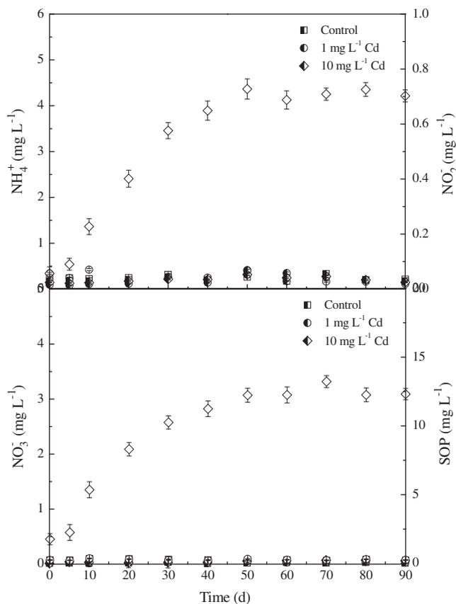
Fig. 3. Effluent concentrations of NH<sub>4</sub><sup>+</sup> (A, white), NO<sub>2</sub><sup>-</sup> (A, half white), NO<sub>3</sub><sup>-</sup> (B, white) and SOP (B, white) during the long-term exposure to no Cd(II), 1 and 10 mg L<sup>-1</sup> Cd(II). Error bars represent standard deviations of triplicate measurements.
