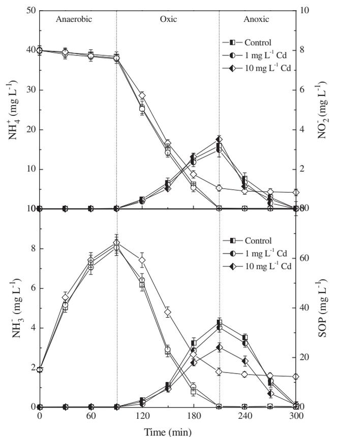
**Fig. 4.** Variations of  $\text{NH}_4^+$  (A, white),  $\text{NO}_2^-$  (A, half white),  $\text{NO}_3^-$  (B, half white) and SOP (B, white) during one cycle after long-term exposure to no Cd(II), 1 and 10 mg L<sup>-1</sup> Cd(II). Error bars represent standard deviations of triplicate measurements.
