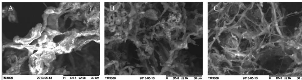
Fig. 1. SEM images of activated sludge exposed to no Cd(II) (control) (A), 1 mg L<sup>-1</sup> (B), and 10 mg L<sup>-1</sup> (C) Cd(II).
