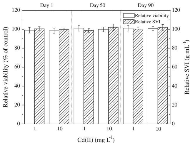
Fig. 2. Effects of 1 and 10 mg L<sup>-1</sup> Cd(II) on relative viability and SVI at day 1, day 50 and day 90. Error bars represent standard deviations of triplicate measurements.
