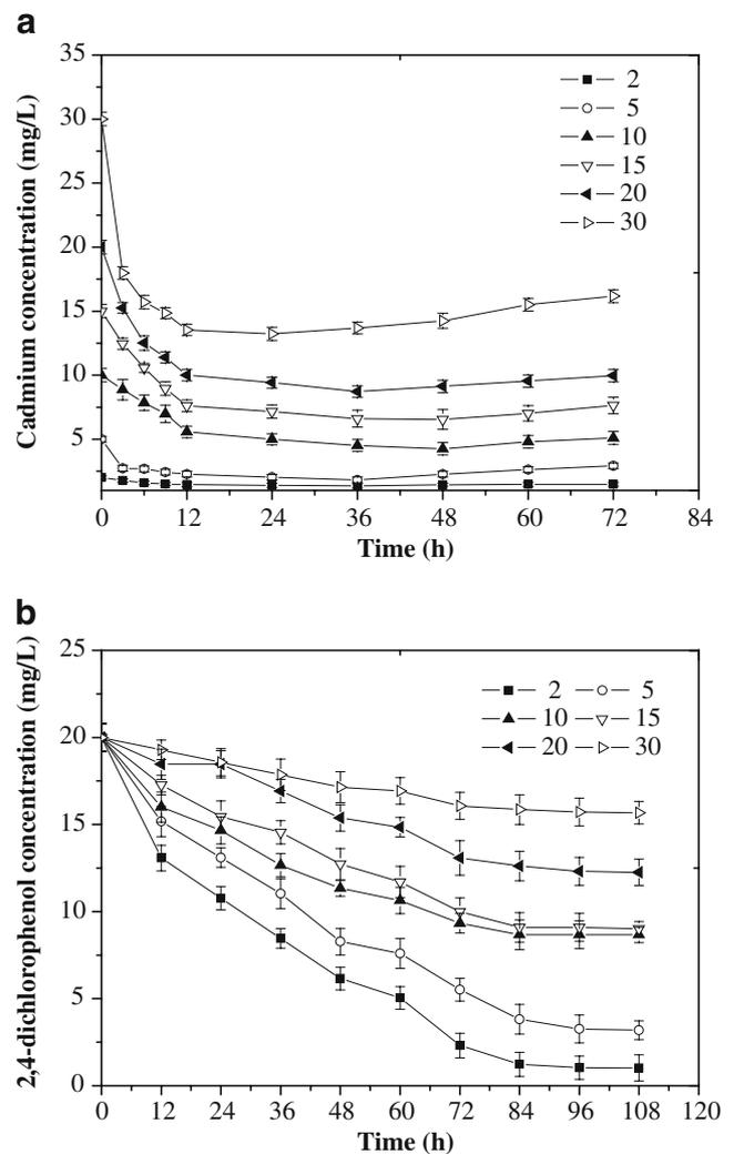
**Fig. 2** Effect of initial cadmium concentration on **a** cadmium removal and **b** 2,4-DCP degradation using *P. chrysosporium* at an initial pH of 6.5 and an initial 2,4-DCP concentration of 20 mg/L; the initial cadmium concentration in the medium was adjusted to 2, 5, 10, 15, 20 and 30 mg/L, respectively
