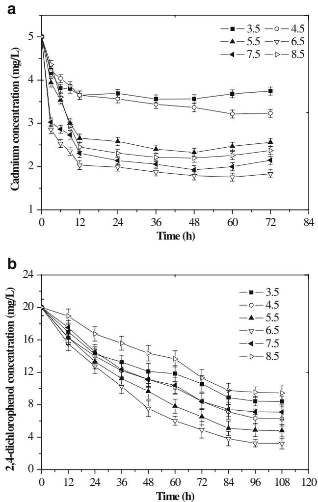
**Fig. 1** Effect of initial pH on **a** cadmium removal and **b** 2,4-DCP degradation using *P. chrysosporium* at an initial cadmium concentration of 5 mg/L and an initial 2,4-DCP concentration of 20 mg/L; the initial pH in the medium was adjusted to 3.5, 4.5, 5.5, 6.5, 7.5 and 8.5, respectively
