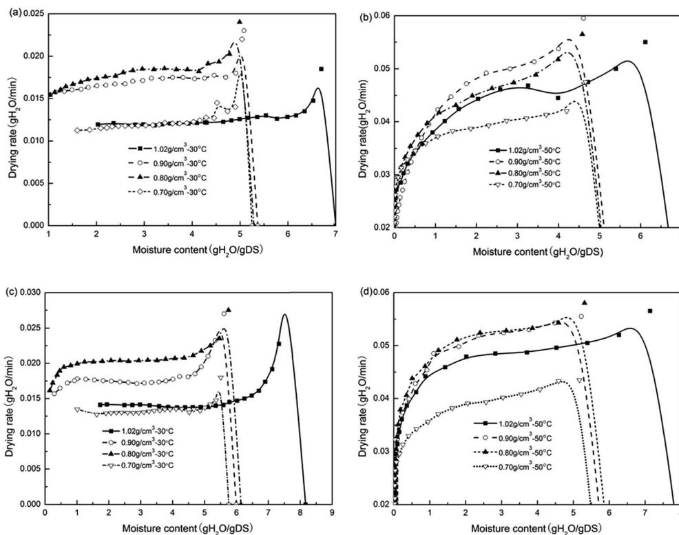
Fig. 6 Relationship between drying rate and drying time of sludge foam-mats at different addition ratios and drying temperatures: (a) 10 g DFS + 10 g CaO, 30 °C; (b) 10 g DFS + 10 g CaO, 50 °C; (c) 20 g CaO, 30 °C; and (d) 20 g CaO, 50 °C (1.02 g cm<sup>-3</sup> was the density of dewatered sludge without the foaming process; 0.90 g cm<sup>-3</sup>, 0.80 g cm<sup>-3</sup> and 0.70 g cm<sup>-3</sup> were the densities of the foamed sludge).
