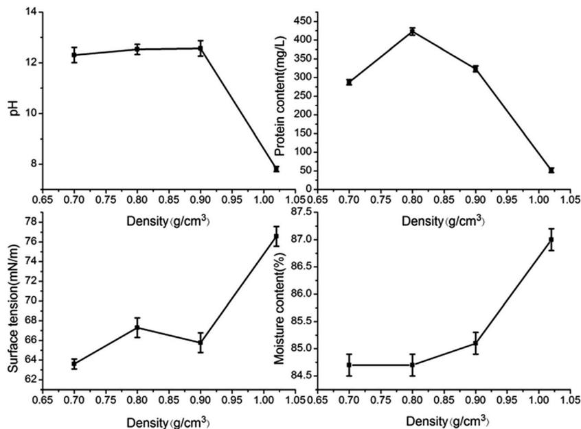
Fig. 7 Effects of back mixing on the protein content, surface tension and pH of the solvent phase of the sludge suspension and the initial moisture content of the sludge foam at different densities (the mass ratio of DFS to CaO is 10 g DFS + 10 g CaO; DFS shape: PDFS; dosing sequence: CaO, then DFS after 5 min).
