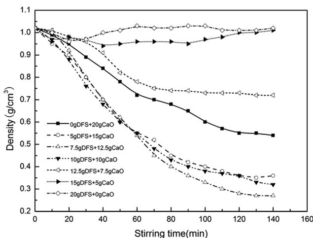
Fig. 1 Effect of stirring time and addition ratios (DFS + CaO) on the sludge foam density (dosing sequence: synchronous addition of DFS and CaO before stirring; DFS shape: PDFS).
