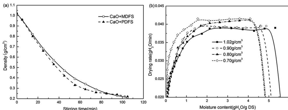
Fig. 4 (a) Effect of DFS shape on the sludge foam density; (b) effect of DFS shape on the drying rate of sludge foam at different densities (the mass ratio of DFS to CaO is 10 g DFS + 10 g CaO; dosing sequence: CaO, then DFS after 5 min; drying temperature: 50 °C).
