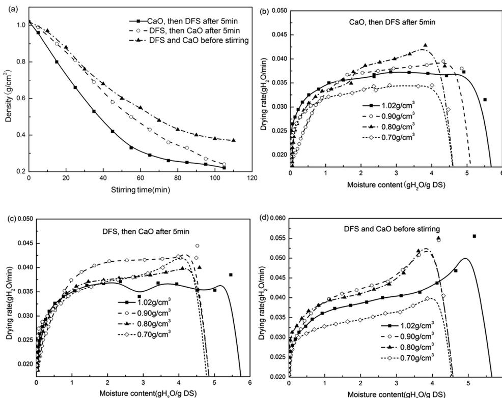
Fig. 3 (a) Effect of different dosing sequences on the sludge foam density; and (b)–(d) effect of different dosing sequences on the drying rate of sludge foam at different densities (the mass ratio of DFS to CaO is 10 g DFS + 10 g CaO; DFS shape: PDFS; and drying temperature: 50 °C).
