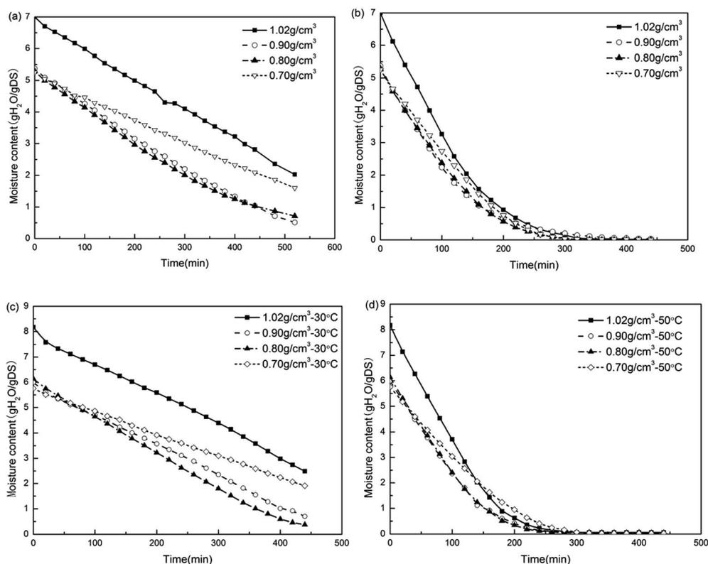
Fig. 5 Drying curves of sludge foam mats at different addition ratios (DFS : CaO) and drying temperatures: (a) 10 g DFS + 10 g CaO, 30 °C; (b) 10 g DFS + 10 g CaO, 50 °C; (c) 20 g CaO, 30 °C; and (d) 20 g CaO, 50 °C (1.02 g cm<sup>-3</sup> was the density of dewatered sludge without the foaming process; and 0.90 g cm<sup>-3</sup>, 0.80 g cm<sup>-3</sup> and 0.70 g cm<sup>-3</sup> were the densities of the foamed sludge).
