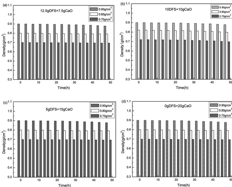
Fig. 2 Variation of sludge foam density over time at different initial densities under the different addition ratios (DFS + CaO) (dosing sequence: synchronous addition of DFS and CaO before stirring; DFS shape: PDFS).
