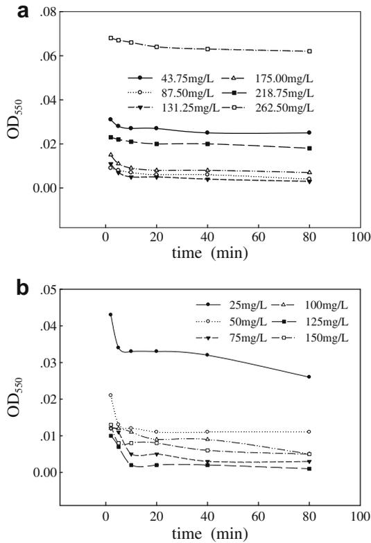
Fig. 1. OD<sub>550</sub> varied with time at different dosage of (a) MBFGA1 and (b) PAC.
