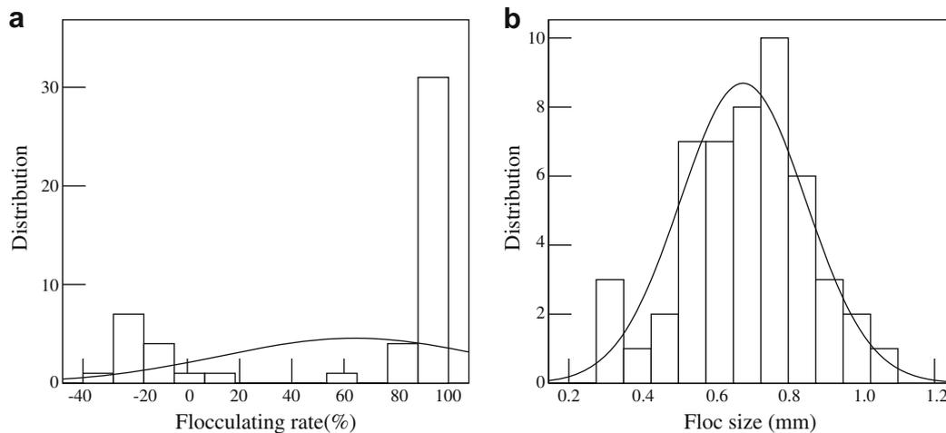
Fig. 4. Distribution of (a) flocculating rate and (b) floc size from the CCD experiment.
