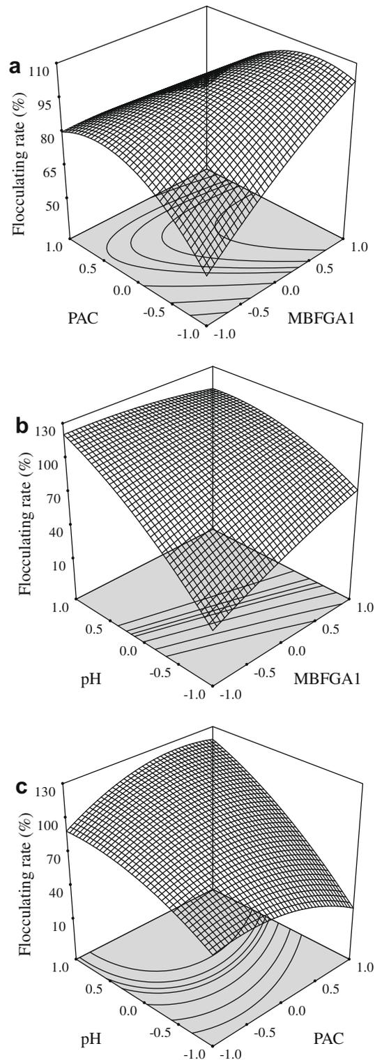
**Fig. 2.** Surface graphs of flocculating rate showing the effect of variables: (a) MBFGA1–PAC, (b) MBFGA1–pH, and (c) PAC–pH.
