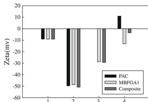
Fig. 5. Contrast of Zeta potential between the flocculants in different time point ((1) kaolin suspension without additives, (2) after adjusting the pH, (3) after adding  $\text{CaCl}_2$ , and (4) after adding the flocculant).
