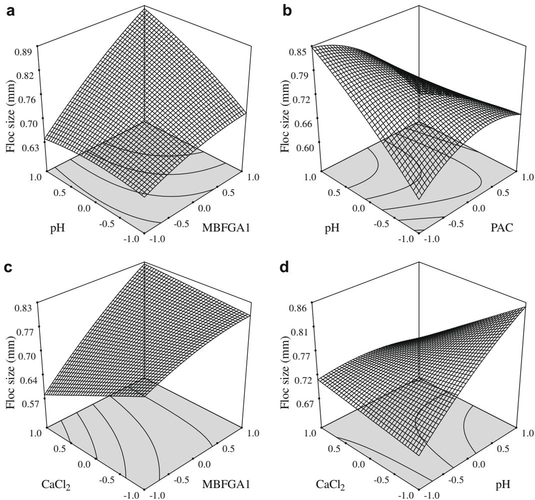
**Fig. 3.** Surface graphs of floc size showing the effect of variables: (a) MBFGA1–pH, (b) PAC–pH, (c) MBFGA1– $\text{CaCl}_2$ , and (d) pH– $\text{CaCl}_2$ .
