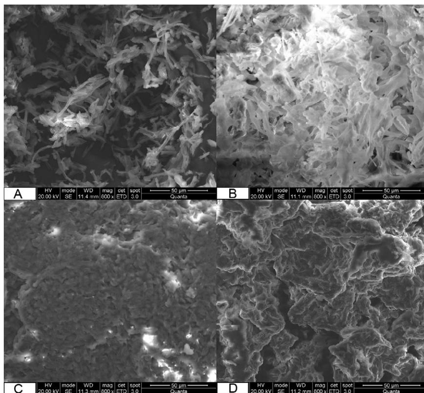
**Fig. 4.** SEM micrographs of *P. simplicissimum*: (A) the intact biomass; (B) the 0.025% saponins-pretreated biomass; (C) the intact biomass after cadmium uptake; (D) the 0.025% saponins-pretreated biomass after cadmium uptake. The adsorption was carried out at pH 5.0 with 20 mg/l Cd(II).
