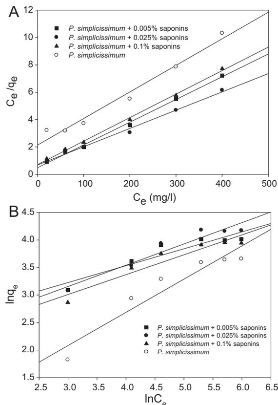
**Fig. 2.** Langmuir isotherms (A) and Freundlich isotherms (B) for Cd(II) biosorption by the intact and saponins-pretreated biomasses. Results are expressed as means of 3 independent measurements and less than 5% standard deviation.
