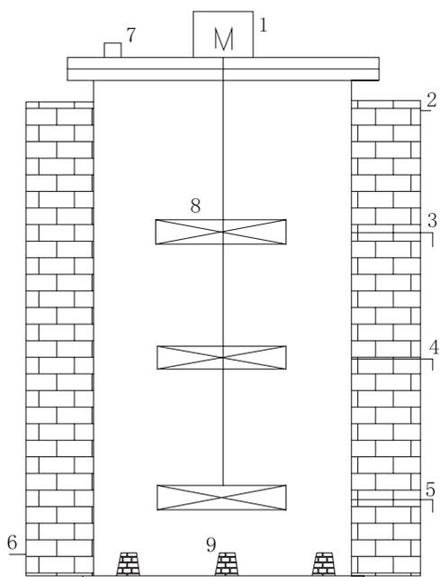
Figure 1. Schematic diagram of S-TE reactor (1: electric stirrer; 2: water exit (water bath layer); 3, 4, 5: sludge exit; 6: water inlet (water bath layer); 7: Sludge inlet; 8: stirrer; 9: air diffuser).
