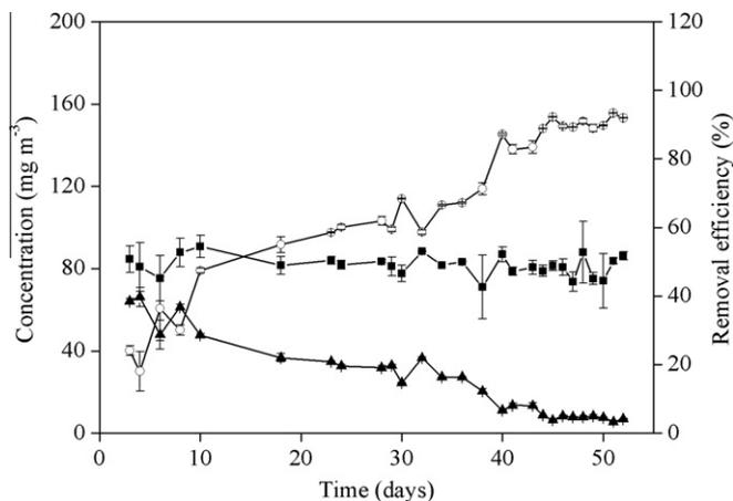
**Fig. 2.** Performance of the tubular biofilter on the startup stage. (■) Inlet toluene concentration, (▲) outlet toluene concentration, (○) toluene removal efficiency. The single data point is representing the mean value of the data, while error bars representing the overall distribution of the data.
