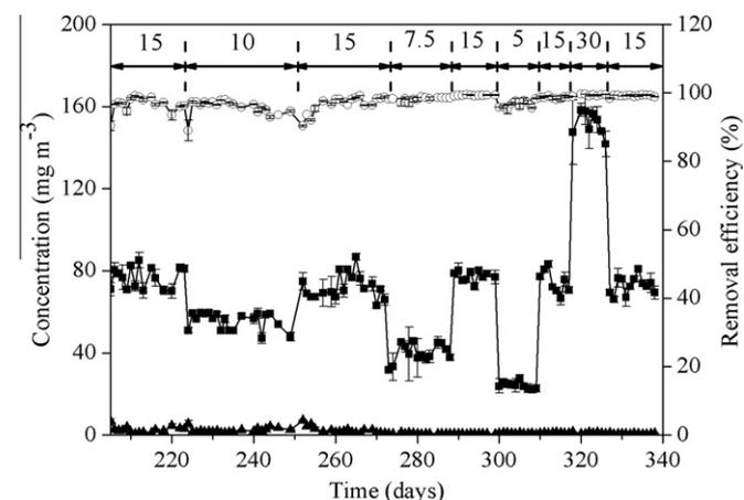
Fig. 4. Toluene removal efficiencies at various gas empty bed residence times and a constant toluene loading rate. (■) Inlet toluene concentration, (▲) outlet toluene concentration, (○) toluene removal efficiency. The single data point is representing the mean value of the data, while error bars representing the overall distribution of the data.
