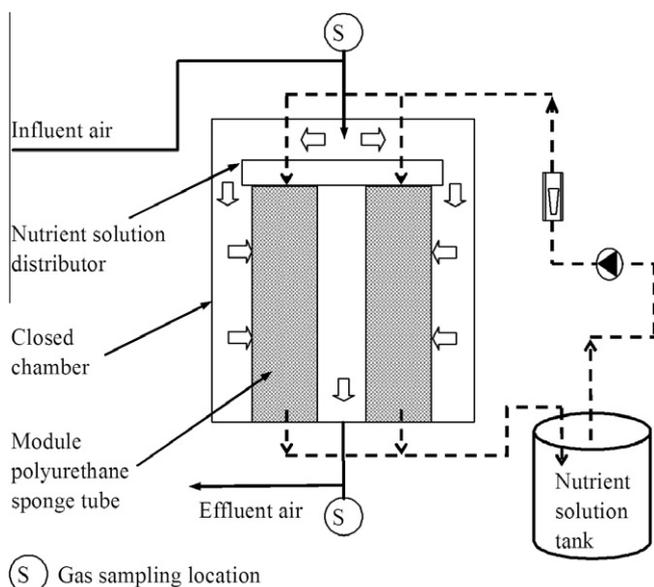
Fig. 1. Schematic of the tubular biofilter.
