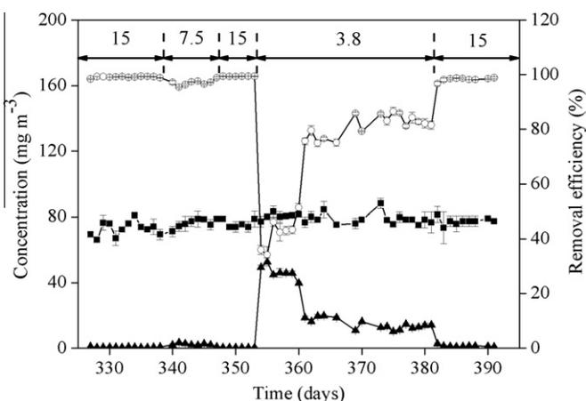
**Fig. 5.** Toluene removal efficiencies at various gas empty bed residence times and a constant incoming pollutant concentration. (■) Inlet toluene concentration, (▲) outlet toluene concentration, (○) toluene removal efficiency. The single data point is representing the mean value of the data, while error bars representing the overall distribution of the data.
