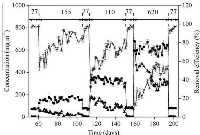
**Fig. 3.** Toluene removal efficiencies at various organic loading rates. (■) Inlet toluene concentration, (▲) outlet toluene concentration, (○) toluene removal efficiency. The single data point is representing the mean value of the data, while error bars representing the overall distribution of the data.
