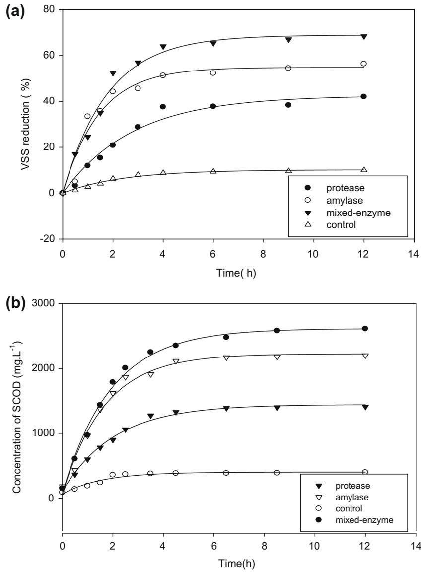
Fig. 5. Variation of VSS reduction and SCOD generation in different enzymes hydrolysis: (a) VSS reduction; and (b) SCOD generation (dosage of enzymes = 6%; protease:amylase = 1:3; hydrolysis temperature = 50 °C).
