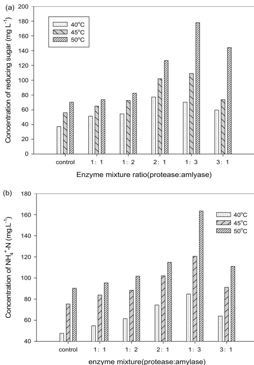
Fig. 4. Variation of reducing sugar and  $\text{NH}_4^+-\text{N}$  concentrations under various enzyme mixture ratio and temperatures: (a) reducing sugar concentration; and (b)  $\text{NH}_4^+-\text{N}$  concentration.
