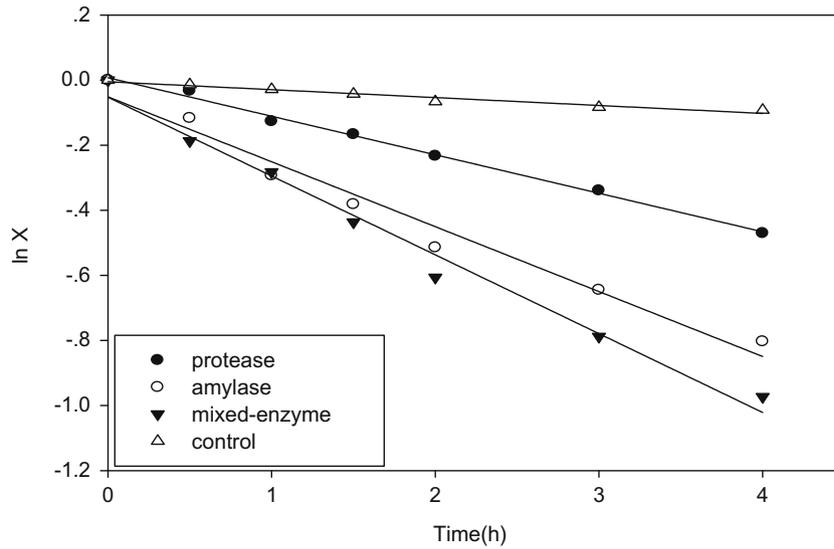
Fig. 6. Relationship between ln X and t during sludge hydrolysis.
