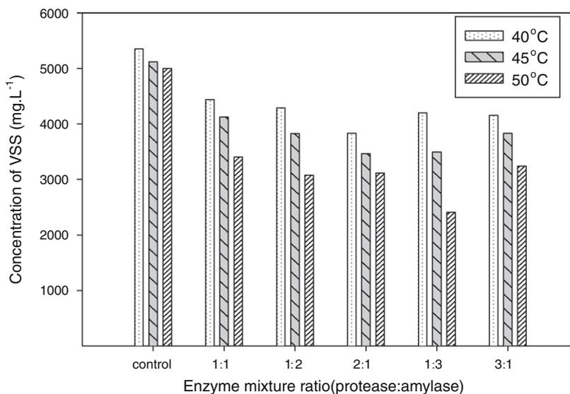
Fig. 3. Effect of temperature and enzyme mixture ratio on enzymatic hydrolysis.
