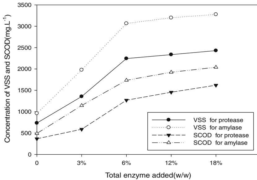
Fig. 2. Effect of single enzyme treatment on solubilisation of excess sludge.
