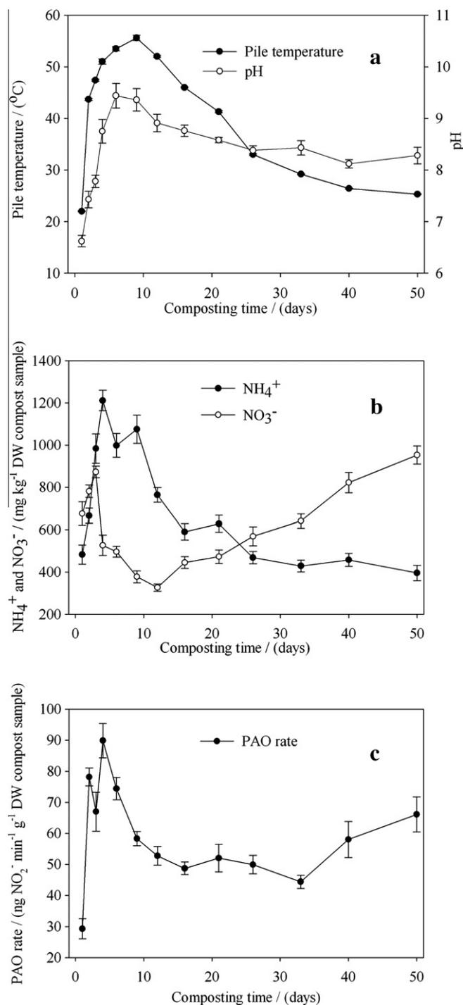
**Fig. 1.** Changes of (a) pile temperature and pH, (b)  $\text{NH}_4^+$  and  $\text{NO}_3^-$ , and (c) PAO rate during agricultural waste composting process. The bars represent the standard deviations of the mean values ( $n = 3$ ).
