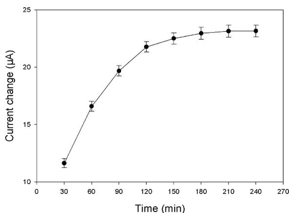
**Fig. 5.** The effects of hybridization time on the SWV peak current change before and after hybridization. The applied concentration of T1 was 0.6 ng/µL. The vertical bars designate the standard deviations for the means of three replicative tests.
