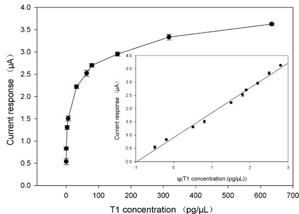
**Fig. 6.** Calibration curves of the sensor response to T1 under the optimal experimental conditions. Inset: linear regression of current response vs. the logarithm of T1 concentration. The vertical bars designate the standard deviations for the means of three replicative tests.
