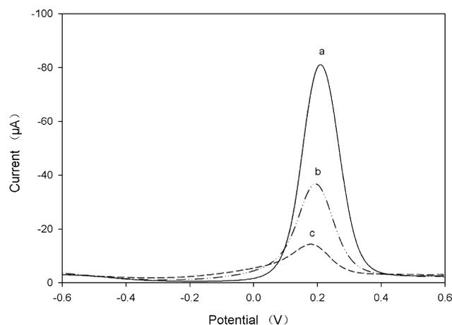
**Fig. 2.** SWVs of different electrodes in a 0.1 M KCl solution containing 5.0 mM ferricyanide. (a) Bare electrode; (b) gold electrode modified with P1 and MPA; (c) the modified gold electrode incubated 2 h in the presence of T1 at 37 °C.
