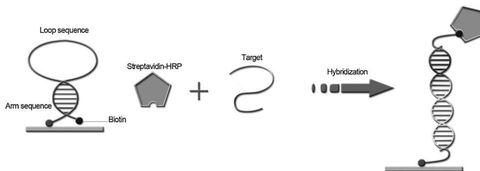
**Fig. 1.** Working principle of the stem-loop structured biosensor. Before hybridization, the probe is closed, when target nucleic acid was captured by the probe, the conformational of the stem-loop structure has changed, triggering the attached biotin group on the electrode surface, binding the streptavidin-horseradish peroxidase (HRP), which produced a electrochemical signal.
