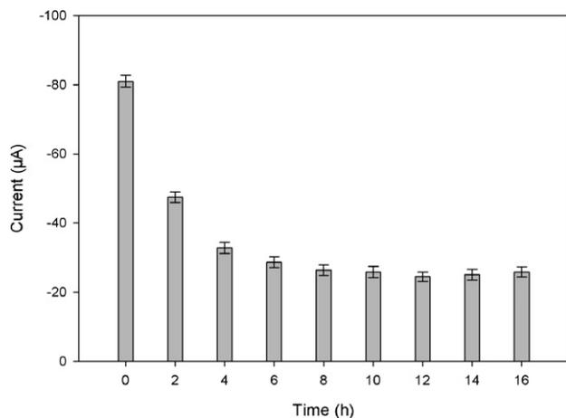
**Fig. 4.** The dependence of peak current of SWVs on self-assembly time of P1 (10 ng/µL) measured in a 0.1 M KCl solution containing 5.0 mM ferricyanide. The vertical bars designate the standard deviations for the means of three replicative tests.
