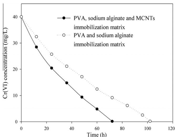
Fig. 4. Cr(VI) reduction by *P. aeruginosa* immobilized in beads with and without multiwalled carbon nanotubes (MWCNTs).
