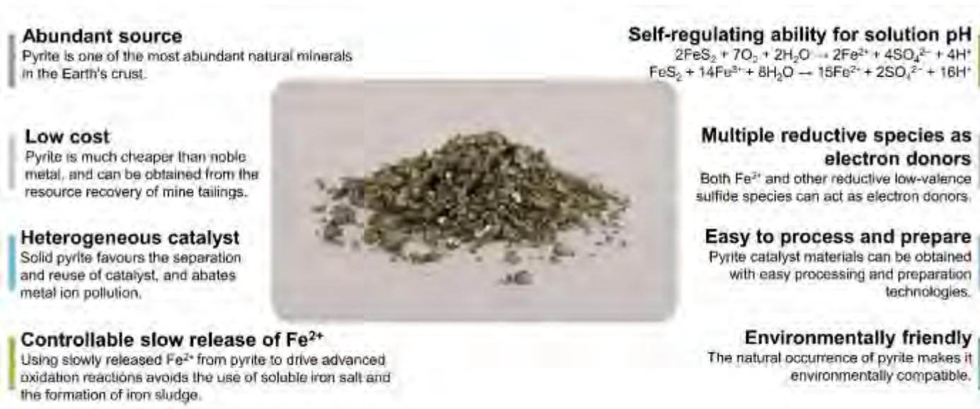
Fig. 6. Main advantages of pyrite as a catalyst for AOPs.
