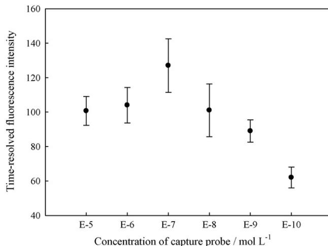
Fig. 2. Optimization of the concentration of capture probe coupling on glass slides. Background signals from blank controls are subtracted.
