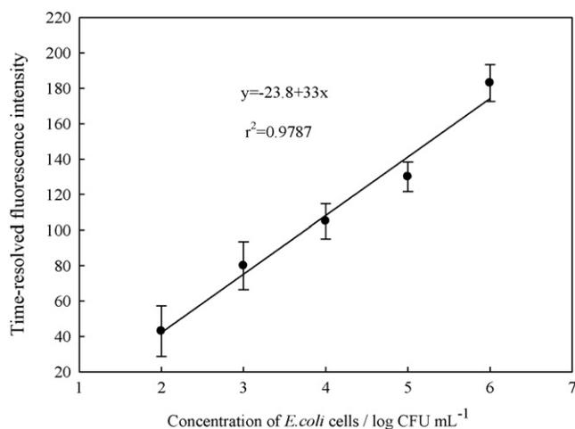
**Fig. 5.** Correlation between fluorescence intensity and the concentration of the *E. coli* cells.
