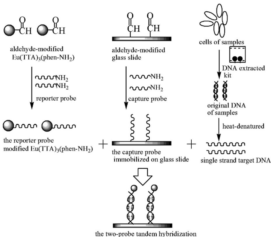
Fig. 1. The schematic diagram of this detection method.
