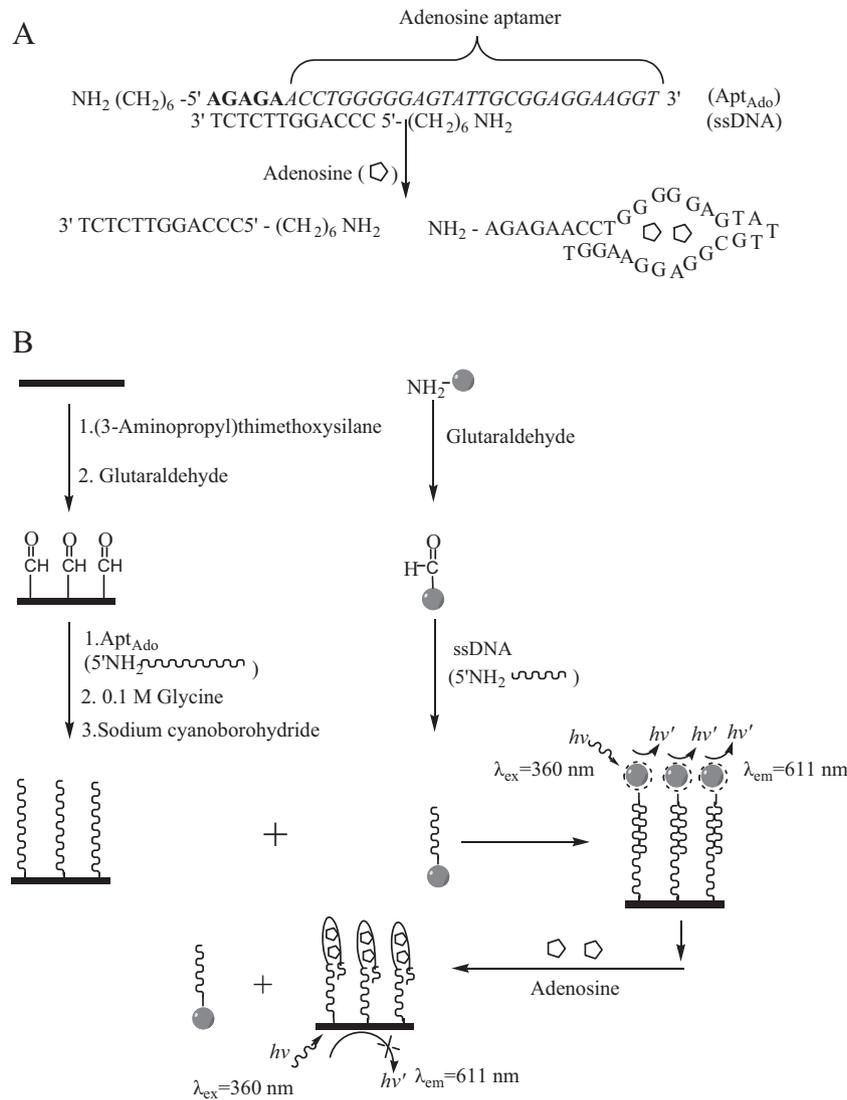
**Scheme 1.** Design of adenosine detection biosensor and the schematic diagram of this method.
