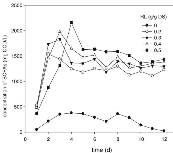
**Fig. 4** Variation of SCFAs concentration with hydrolysis time under different rhamnolipid dosages
