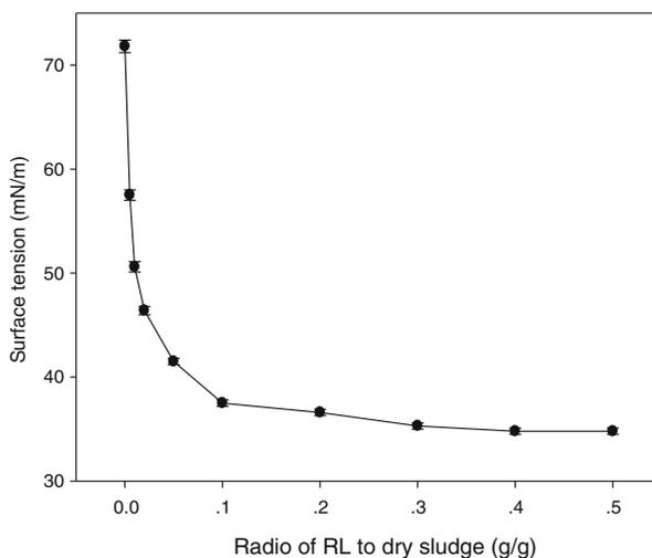
**Fig. 6** Effect of RL on the surface tension at different rhamnolipid dosages
