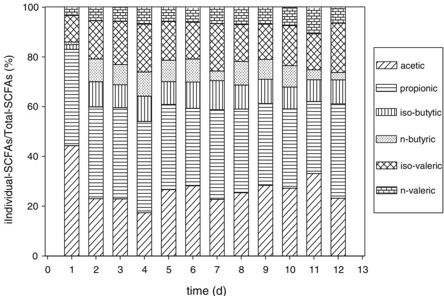
**Fig. 5** Profiles of individual SCFAs concentration during the entire fermentation at RL 0.3 g/g
