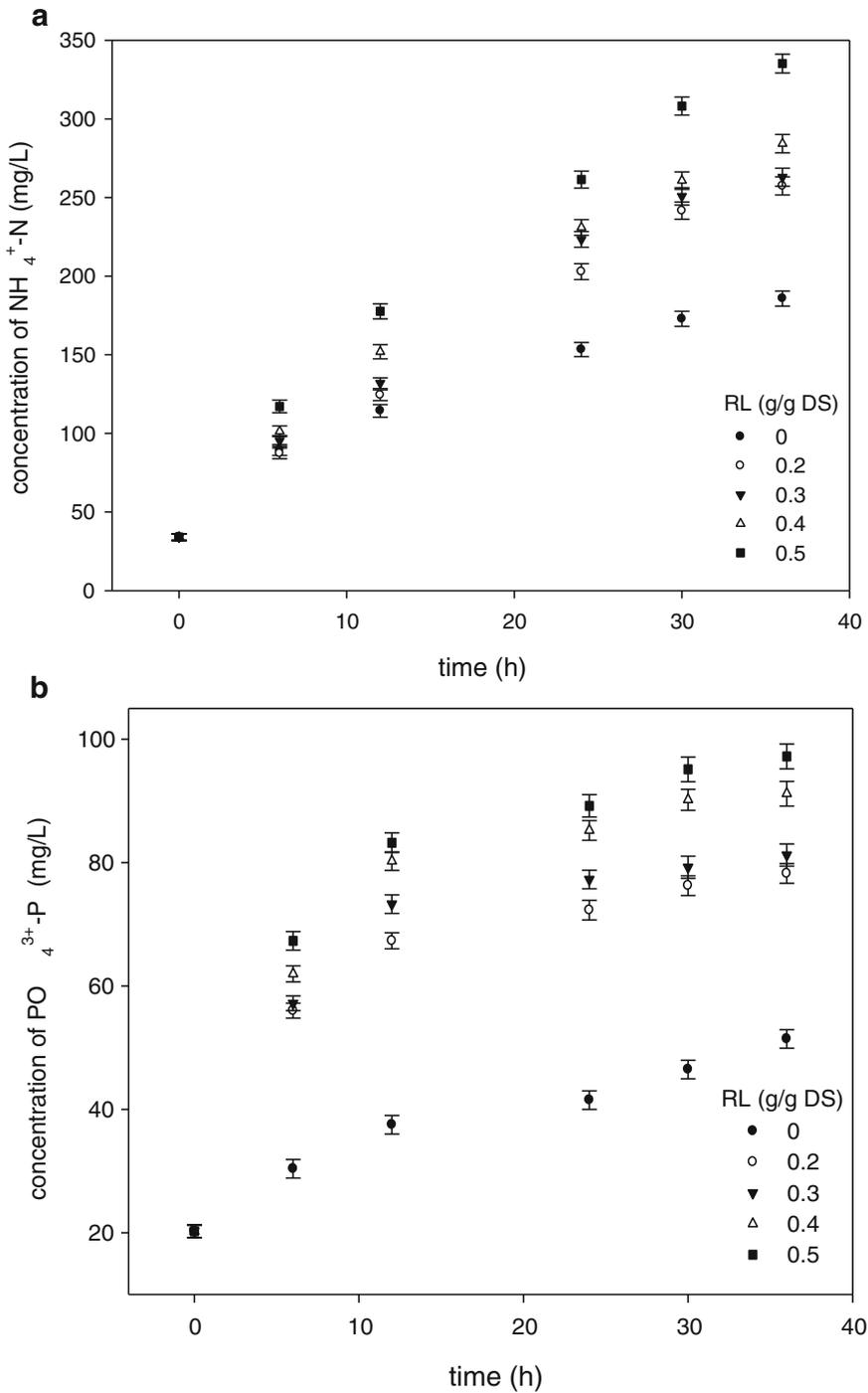
**Fig. 3** Variation of  $\text{NH}_4^+\text{-N}$  and  $\text{PO}_4^{3-}\text{-P}$  concentration with hydrolysis time under different rhamnolipid dosages: **a**  $\text{NH}_4^+\text{-N}$  concentration; **b**  $\text{PO}_4^{3-}\text{-P}$  concentration
