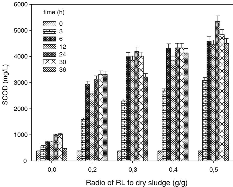
**Fig. 1** Effect of RL on SCOD concentration at different fermentation times
