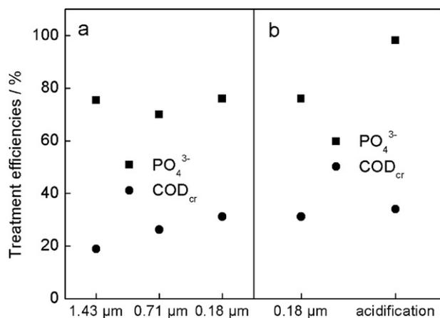
**Fig. 1.** COD<sub>cr</sub> and PO<sub>4</sub><sup>3-</sup> removal efficiencies by employing honeycomb cinders with particle sizes of 0.71–1.43 μm (A), 0.18–0.71 μm (B), less than 0.18 μm (C). Less than 0.18 μm (D) after acidified. Experimental conditions: pH of 8.8, temperature of 30 °C, honeycomb cinders dose of 10.0 g L<sup>-1</sup>, reaction time of 20 min and settling time of 20 min (the conditions of this experiment were selected on the basis of previous experiments).
