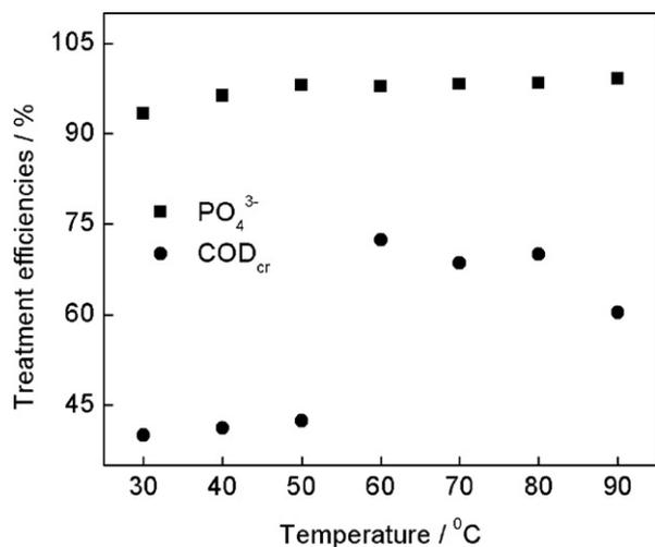
**Fig. 5.** Temperature effect on  $\text{COD}_{\text{cr}}$  and  $\text{PO}_4^{3-}$  removal efficiencies, respectively. Experimental conditions: pH of 5.0, modified honeycomb cinders dose of 10.0 g L<sup>-1</sup>, reaction time of 20 min and settling time of 20 min.
