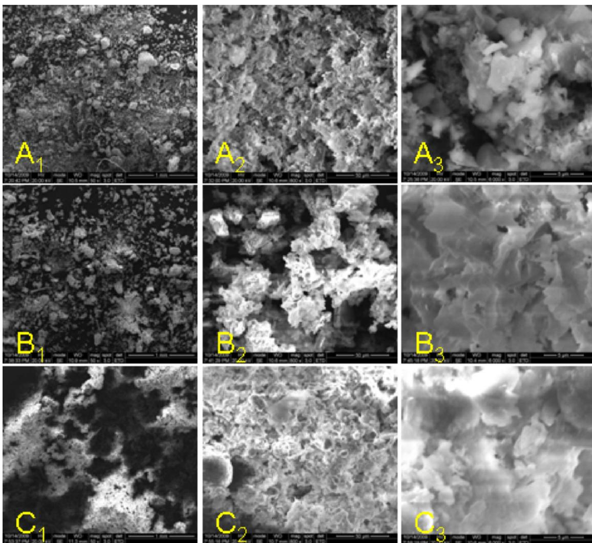
**Fig. 2.** SEM images of raw (A<sub>1</sub>–A<sub>3</sub>) and modified (B<sub>1</sub>–B<sub>3</sub>) honeycomb cinders with various resolutions of 1 mm, 50 μm, 5 μm, and of the resulting precipitates (C<sub>1</sub>–C<sub>3</sub>).
