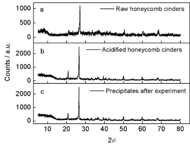
Fig. 3. XRD analysis of raw (a) and modified (b) honeycomb cinders, and resulting precipitates (c).
