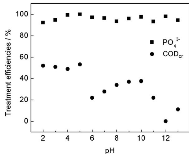
Fig. 4. pH effect on  $\text{COD}_{\text{cr}}$  and  $\text{PO}_4^{3-}$  removal efficiencies, respectively. Experimental conditions: temperature of 30 °C, modified honeycomb cinders dose of 10.0 g L<sup>-1</sup>, reaction time of 20 min and settling time of 20 min.
