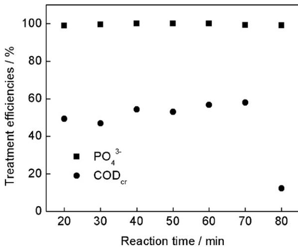
Fig. 7. COD<sub>cr</sub> and PO<sub>4</sub><sup>3-</sup> removal efficiencies under various reaction times. Experimental conditions: pH of 5.0, temperature of 60 °C, modified honeycomb cinders dose of 30.0 g L<sup>-1</sup>, and settling time of 20 min.
