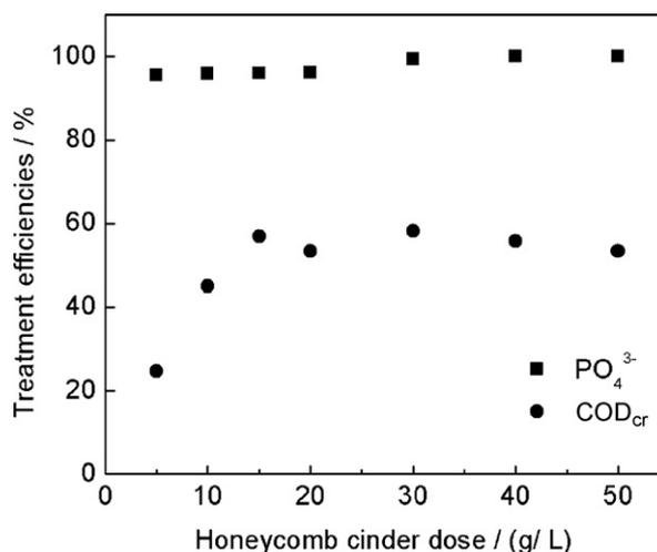
**Fig. 6.** Removal efficiencies of  $\text{COD}_{\text{cr}}$  and  $\text{PO}_4^{3-}$  under various dosages of modified honeycomb cinders. Experimental conditions: pH of 5.0, temperature of 60 °C, reaction time of 20 min and settling time of 20 min.
