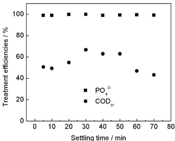
Fig. 8. Removal efficiencies of COD<sub>cr</sub> and PO<sub>4</sub><sup>3-</sup> under various settling time. Experimental conditions: pH of 5.0, temperature of 60 °C, modified honeycomb cinders dose of 30.0 g L<sup>-1</sup>, reaction time of 25 min.
