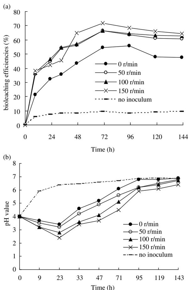
Figure 3. (a) Influence of the incubator rotation speeds on bioleaching ratio, where data measured at min 0 represent the value that was obtained at the beginning of the experiment, and the initial concentration of  $Mn^{2+}$  was 0. (b) The variation of pH value during the bioleaching process.
