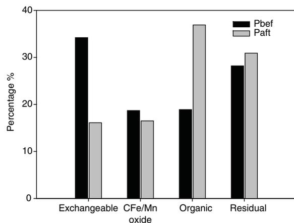
Figure 6. Form percentage of Mn<sup>2+</sup> before and after bioleaching; the initial concentrations of Mn<sup>2+</sup> before and after bioleaching were 35,450 mg/kg and 10,067.8 mg/kg, respectively.
