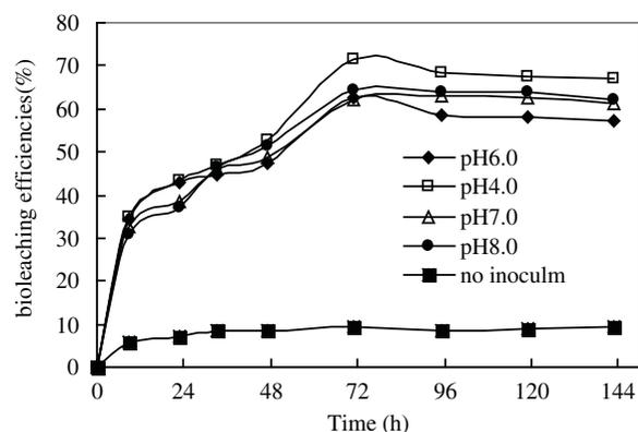
Figure 4. Effect of the initial pH value on manganese bioleaching rate, where data measured at min 0 represent the value that was obtained at the beginning of the experiment, and the initial concentration of  $Mn^{2+}$  was 0.
