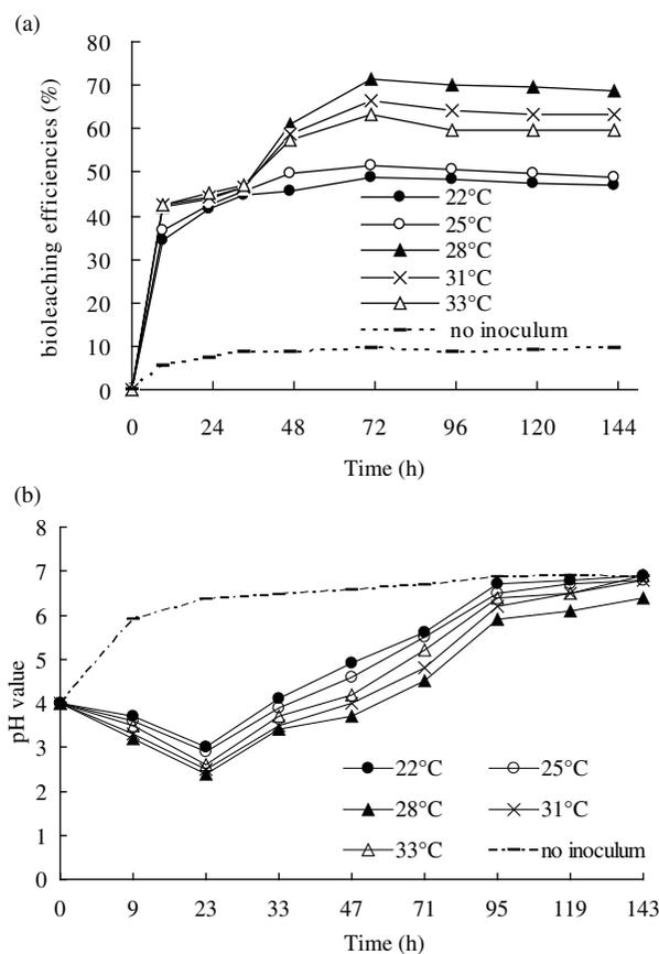
Figure 2. (a) Effect of temperature on  $Mn^{2+}$  bioleaching rate, where data measured at min 0 represents the value that was obtained at the beginning of the experiment, and the initial concentration of  $Mn^{2+}$  was 0. (b) The variation of pH value during the bioleaching process.
