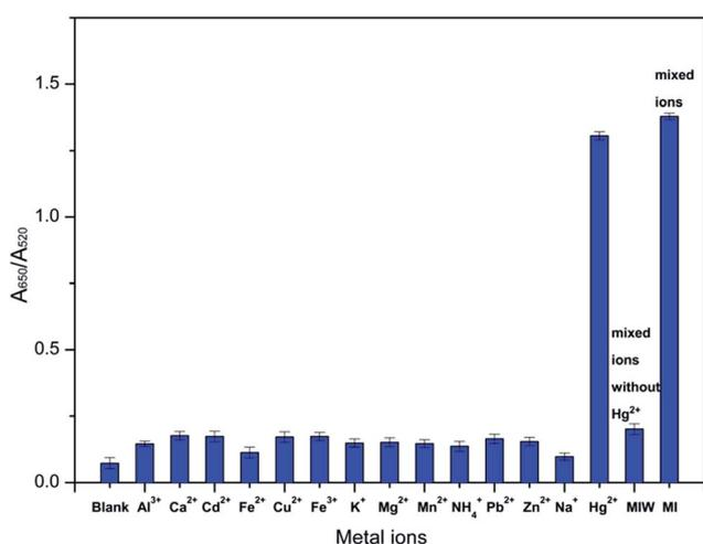
Fig. 5 Ratio values of A<sub>650</sub>/A<sub>520</sub> for P-PDCA-AuNPs versus the different kinds of ions. Concentration of Hg<sup>2+</sup> was 1 mM, while others were 20 mM. Error bars were obtained from three experiments.
