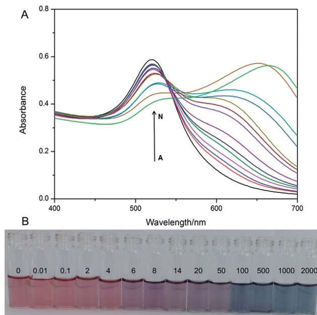
Fig. 3 (A) UV-Vis absorption spectra of P-PDCA-AuNPs were in the presence of different concentrations of  $\text{Hg}^{2+}$  (A to N express 2000, 1000, 500, 100, 50, 20, 14, 8, 6, 4, 2, 0.1, 0.01, 0  $\mu\text{M}$ , respectively). (B) Images of P-PDCA-AuNPs containing different concentrations of  $\text{Hg}^{2+}$  (0, 0.01, 0.1, 2, 4, 6, 8, 14, 20, 50, 100, 500, 1000, 2000  $\mu\text{M}$ ).
