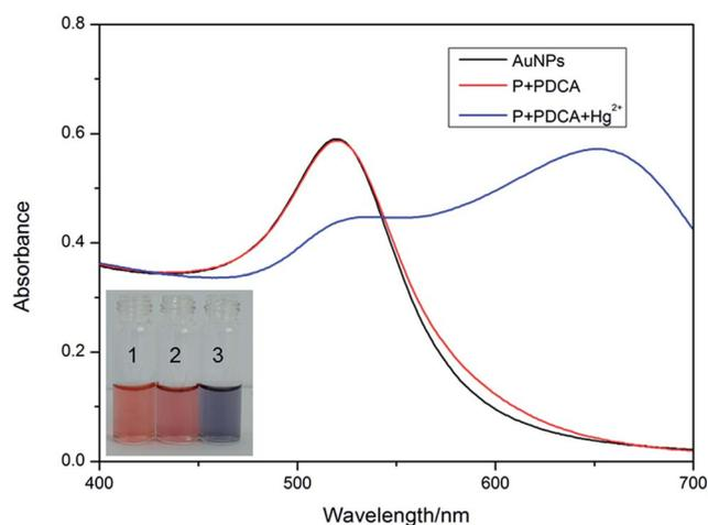
Fig. 1 UV-Vis absorption spectra of the AuNPs (13 nm), P-PDCA-AuNPs (13 nm), and P-PDCA-AuNPs (13 nm) in the presence of 1 mM of  $\text{Hg}^{2+}$ . Inset shows the color change versus the (1) AuNPs (13 nm), (2) P-PDCA-AuNPs (13 nm), and (3) P-PDCA-AuNPs (13 nm) in the presence of 1 mM of  $\text{Hg}^{2+}$ .
