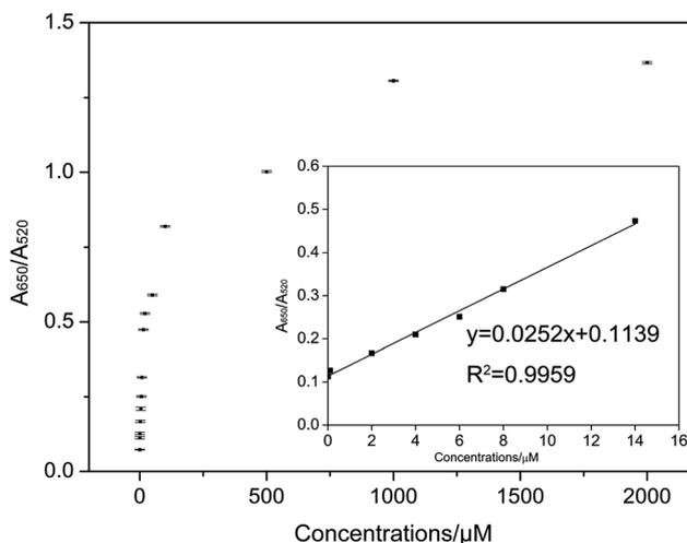
Fig. 4 Ratio values of  $A_{650}/A_{520}$  for P-PDCA-AuNPs versus the concentrations of  $\text{Hg}^{2+}$  (0, 0.01, 0.1, 2, 4, 6, 8, 14, 20, 50, 100, 500, 1000, 2000  $\mu\text{M}$ ). Image of insert is the linear correlation. Error bars were obtained from three experiments.
