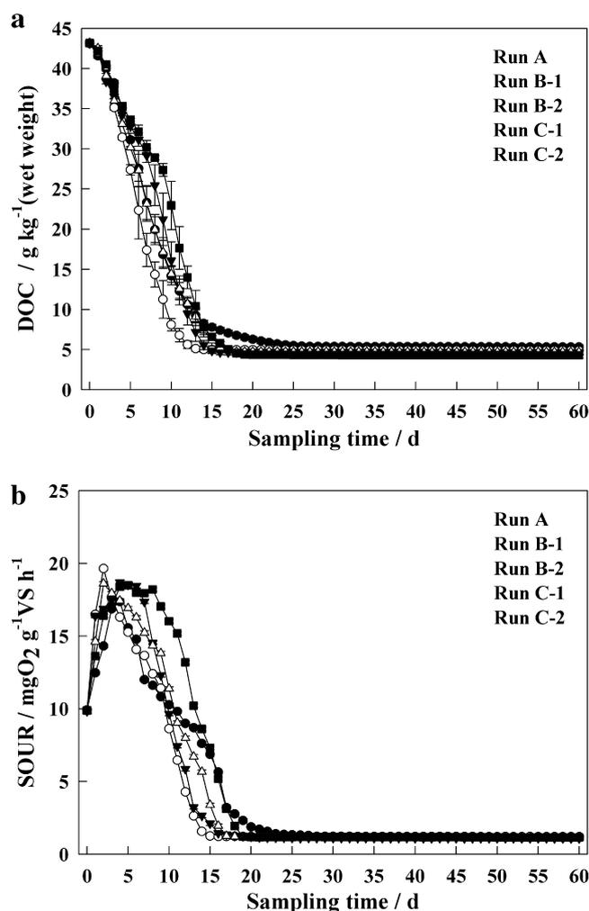
Fig. 4. Daily changes of dissolved organic carbon (DOC) (a) and specific oxygen uptake rate (SOUR) (b) in the five triplicated runs.
