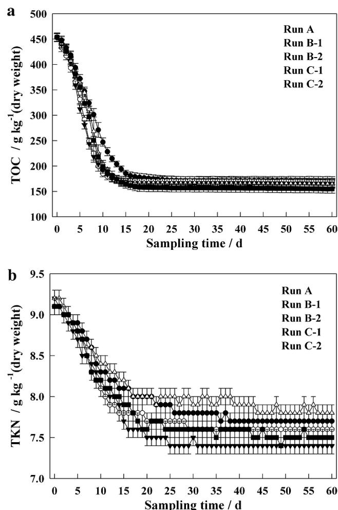
Fig. 2. Daily changes of total organic carbon (TOC) (a) and total Kjeldahl nitrogen (TKN) (b) in the five triplicated runs.
